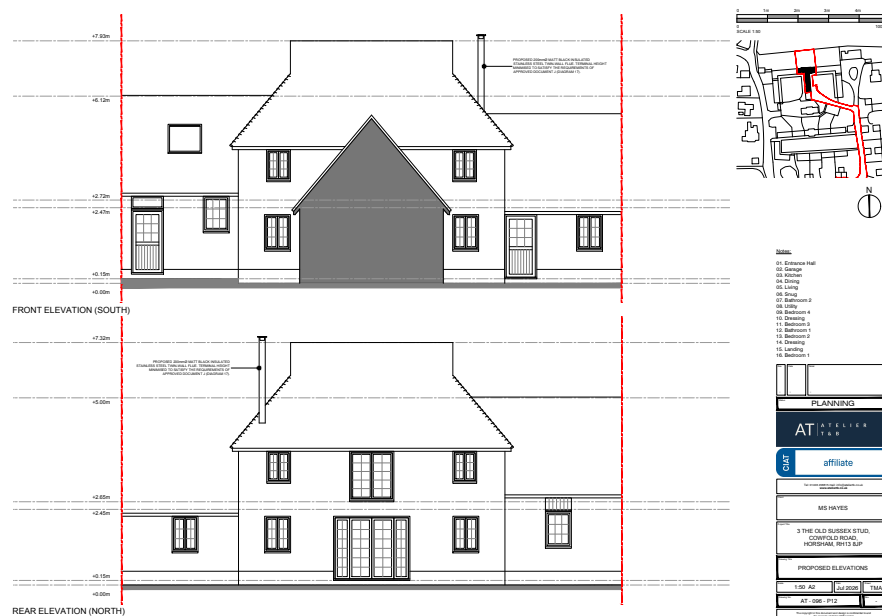
Figure 3 – Proposed elevation illustrating the position and height of the external insulated twin-wall flue.
