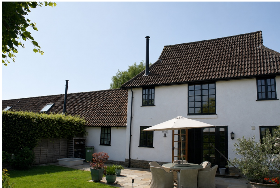
Figure 4 – Photomontage illustrating the proposed external twin-wall flue in its intended location
