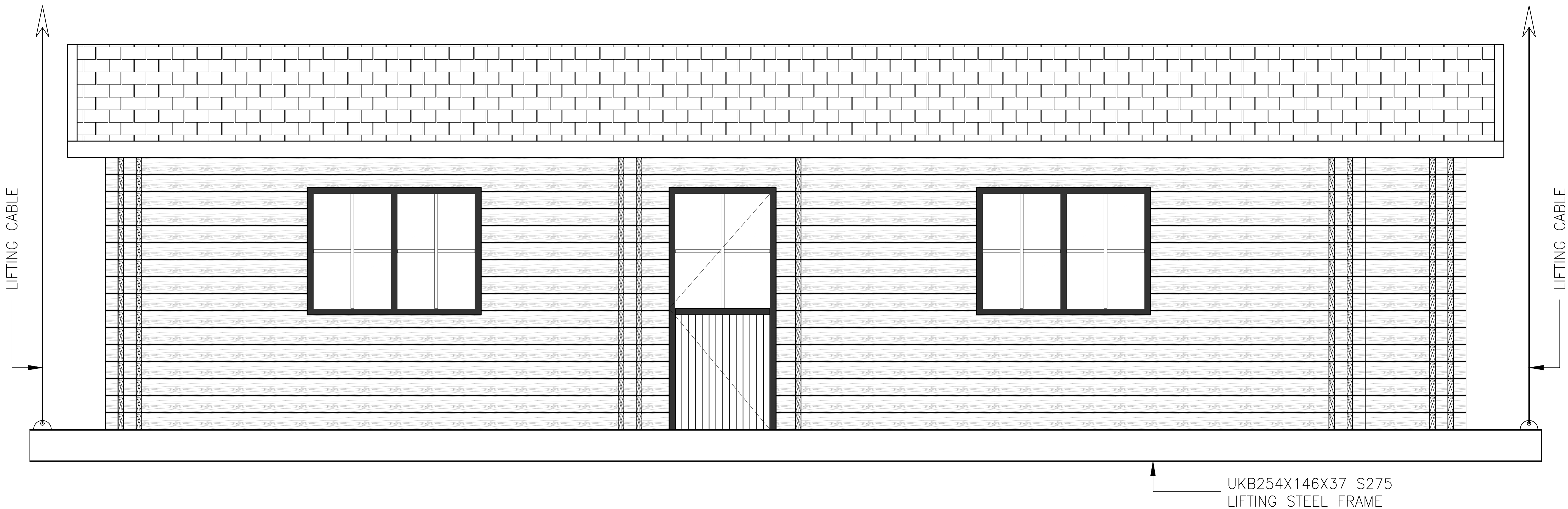
LIFTING ELEVATION (LONGITUDINAL VIEW) SCALE 1:40M
