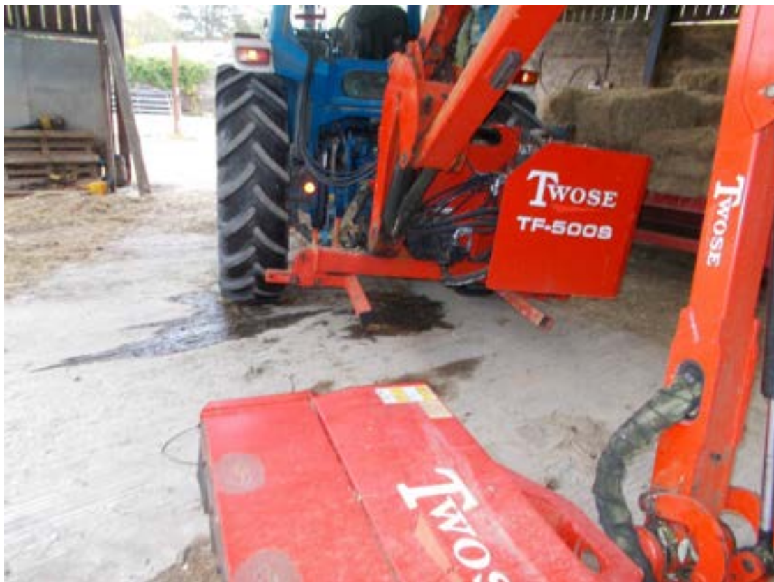
Oil staining beneath tractor
