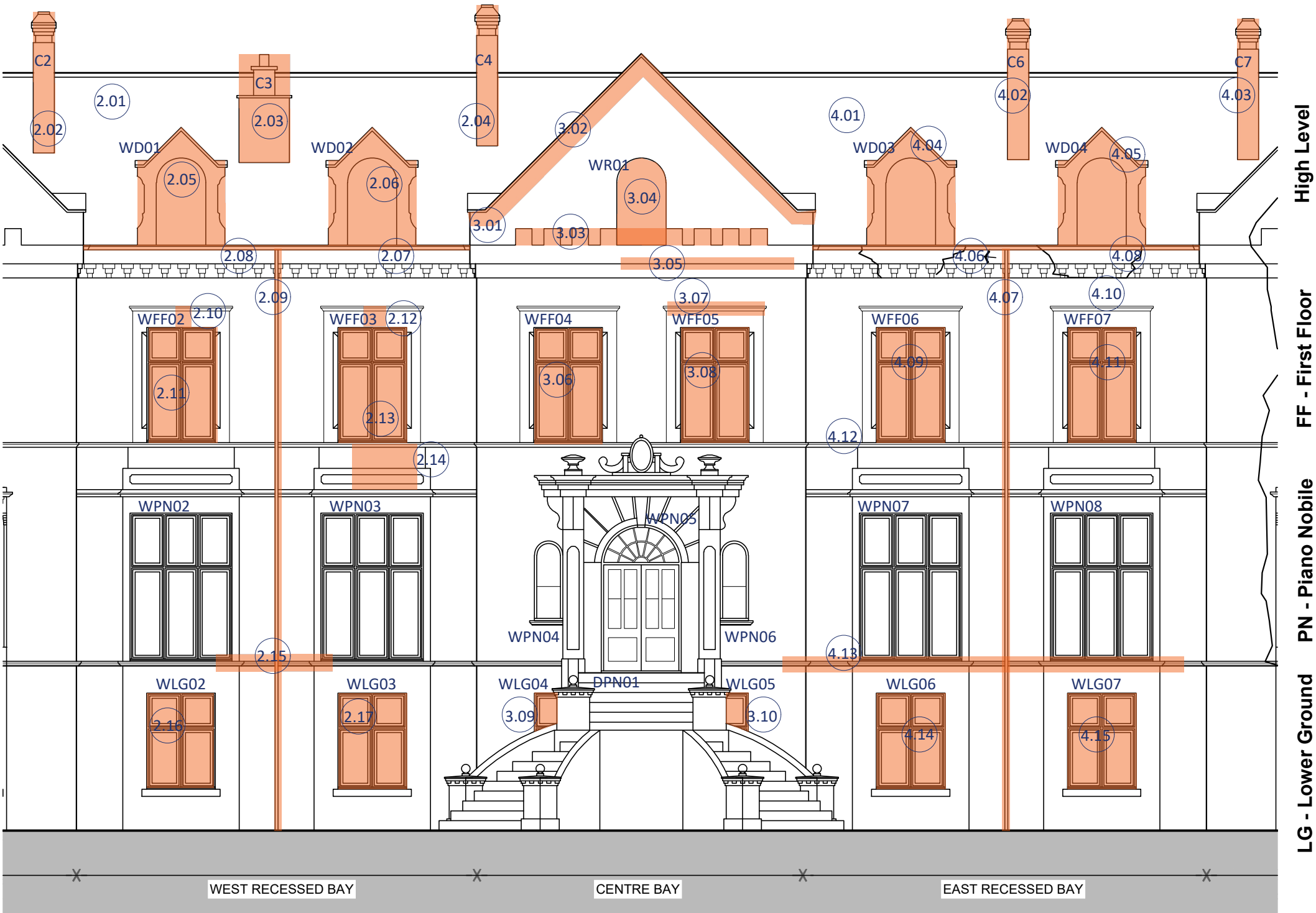
South Elevation, Central - Proposed Repairs
