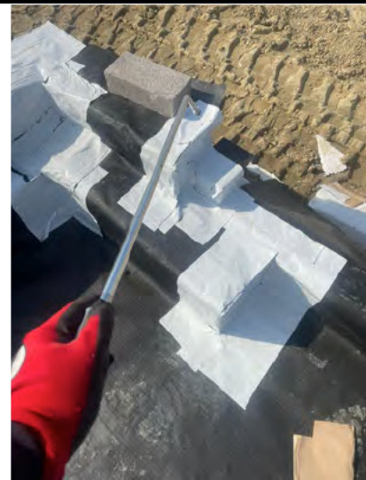
Air lance test on a corner.
