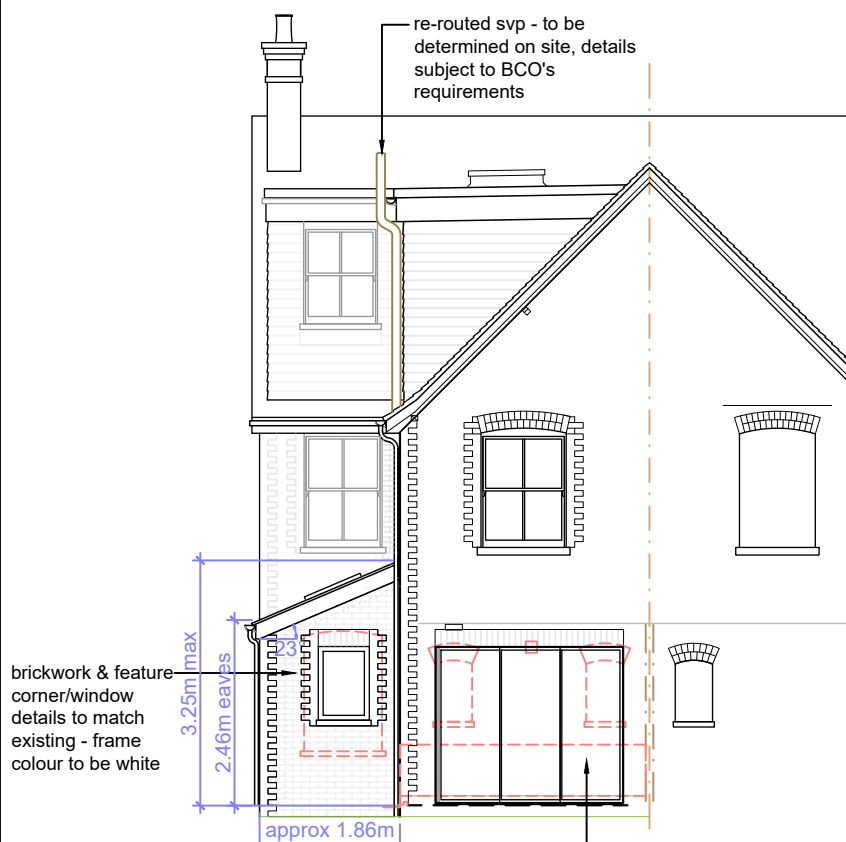
rear (North) elevation
