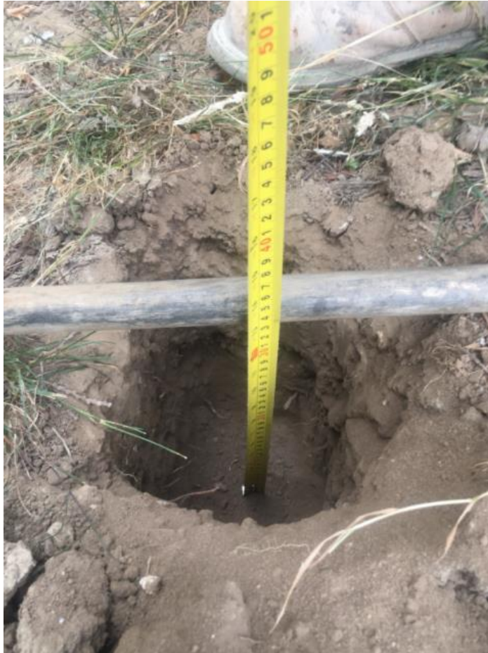
Total Depth of Trial Hole (340 mm)
