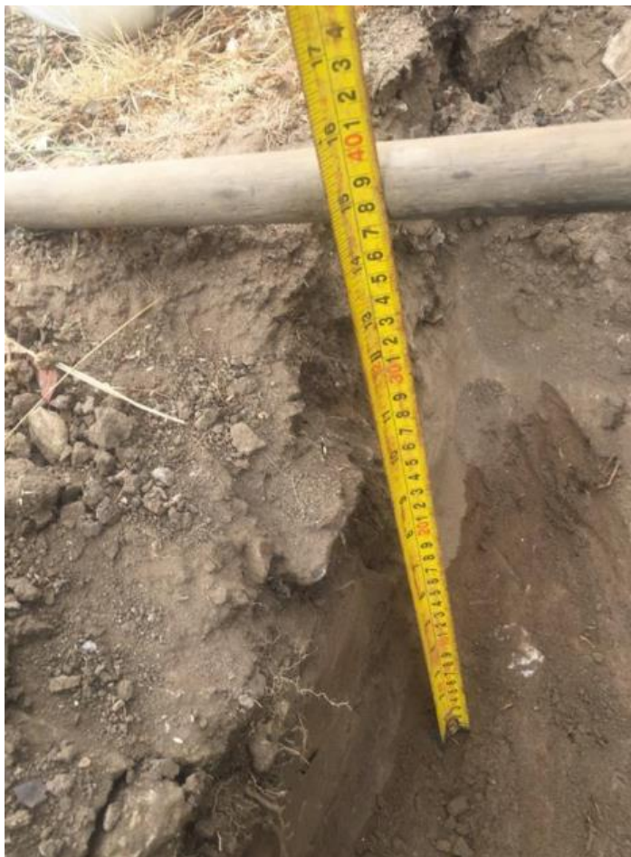
Total Depth of Trial Hole (370 mm)
