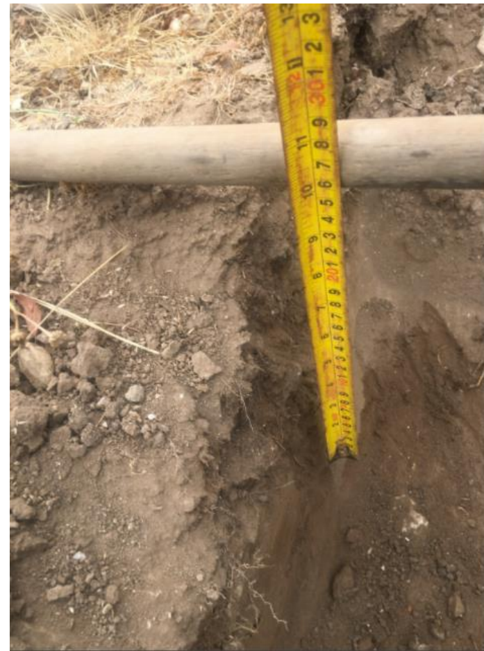
Thickness of Topsoil (260 mm)
