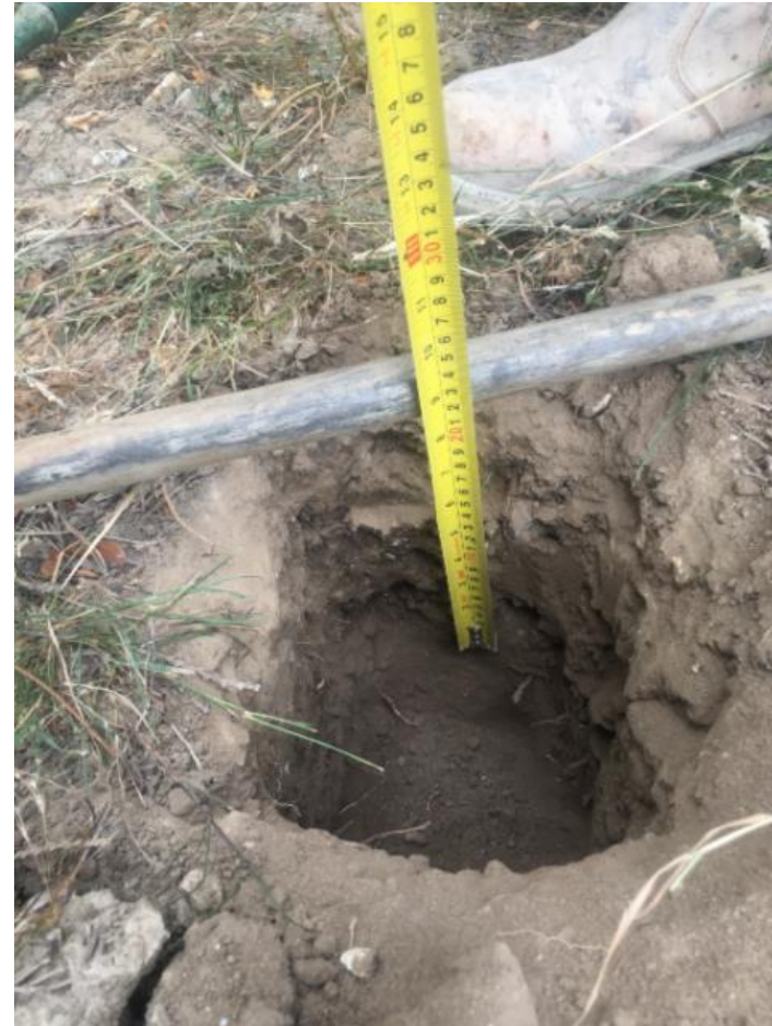
Thickness of Topsoil (220 mm)
