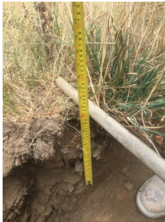
Thickness of Topsoil (300 mm)
