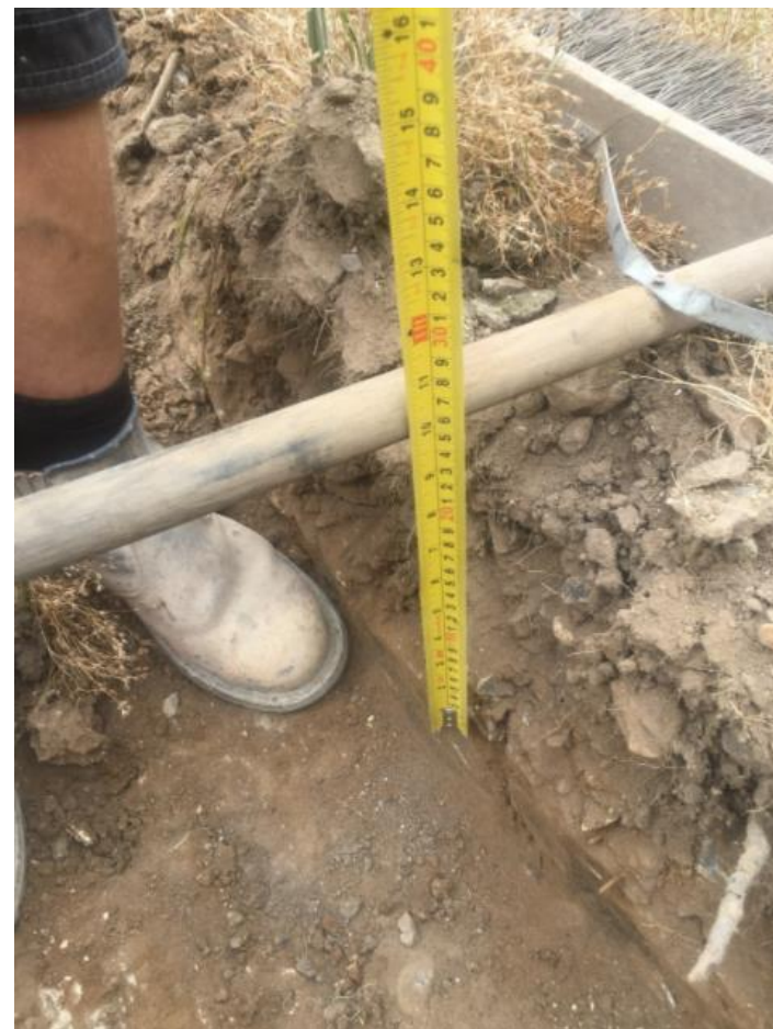
Thickness of Topsoil (260 mm)
