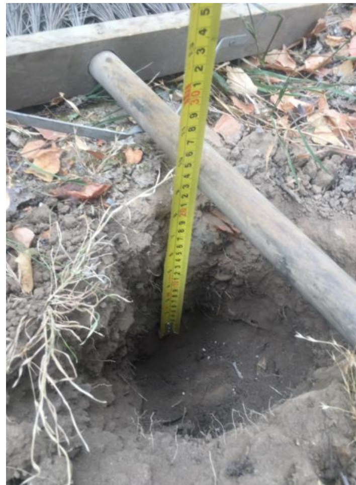
Thickness of Topsoil (230 mm)
