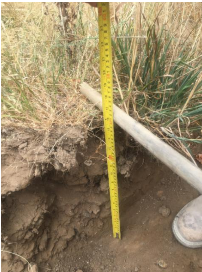
Total Depth of Trial Hole (410 mm)
