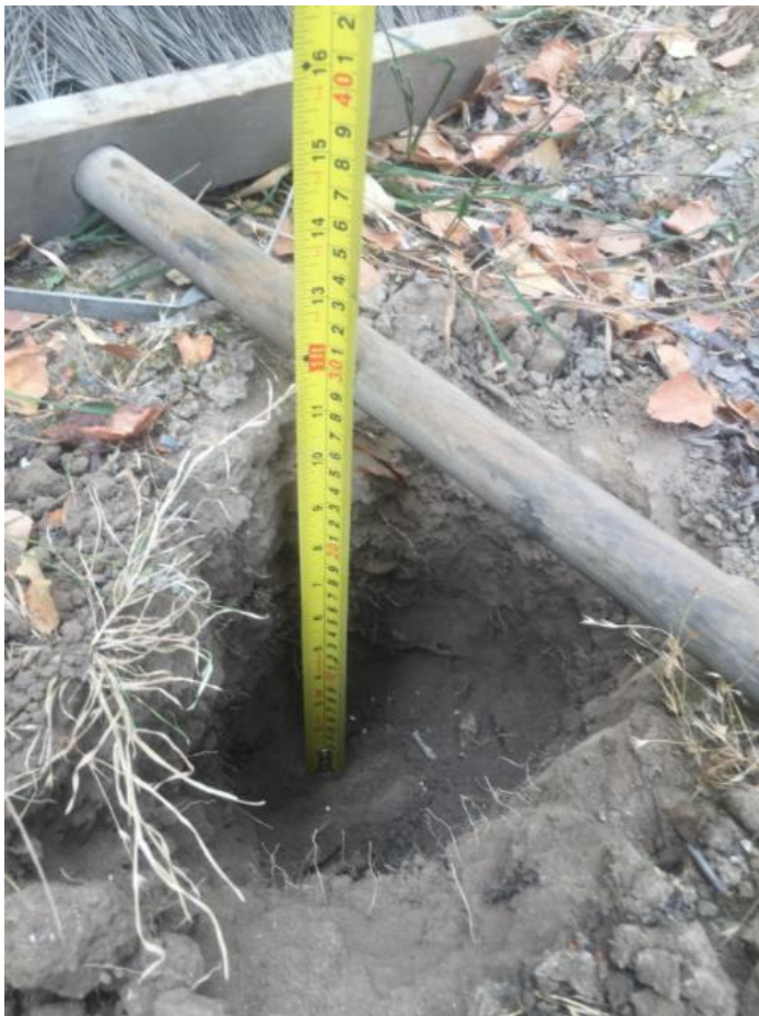
Total Depth of Trial Hole (290 mm)
