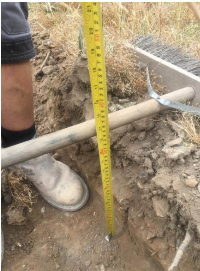
Total Depth of Trial Hole (350 mm)
