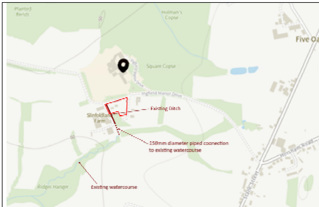
Figure 6 – Surface Water Ditches shown Green
