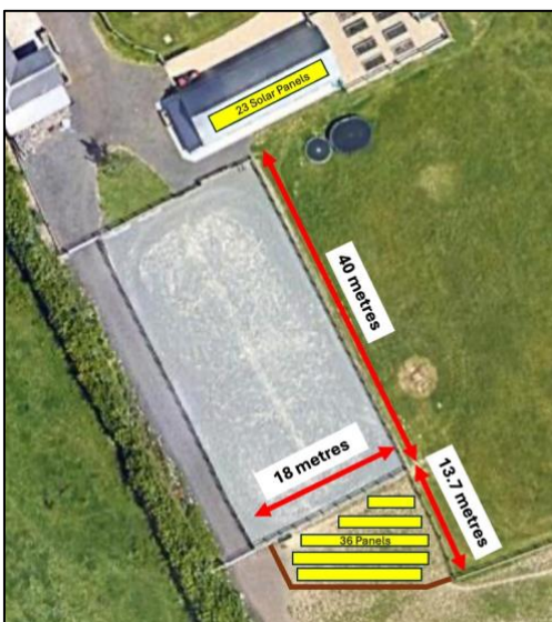
36 solar panel location in relation to the rest of solar equipment location
