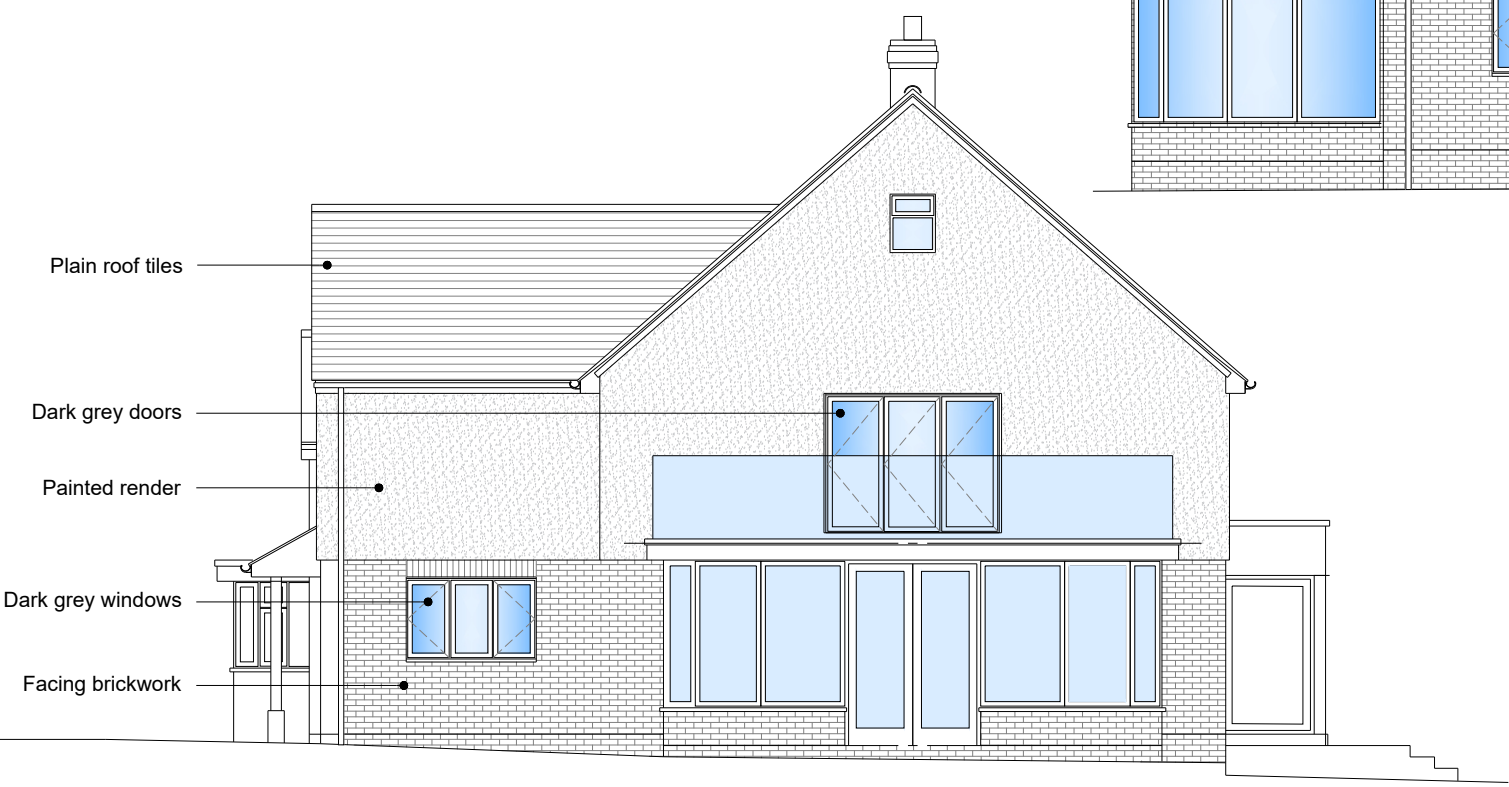
EXISTING SIDE ELEVATION (North East)
