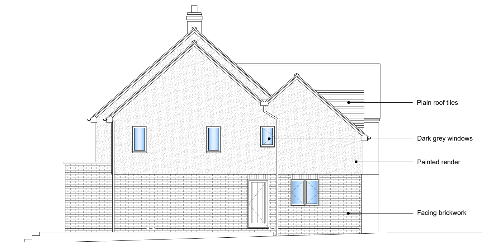
EXISTING SIDE ELEVATION (South West)
