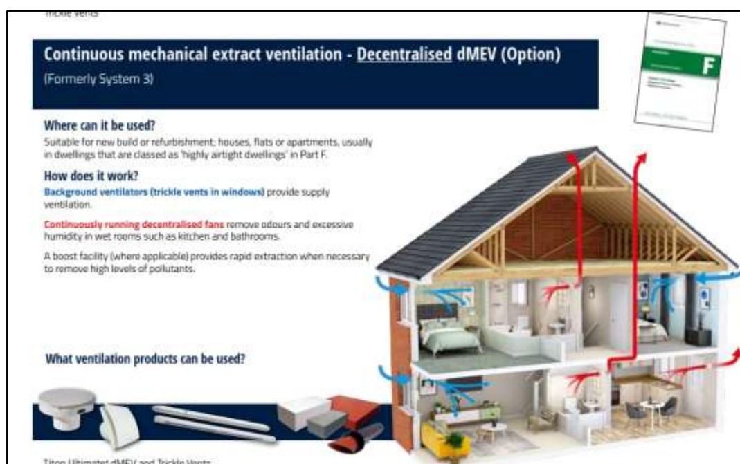
Figure 4. Example of dMEV from Titon Catalogue
