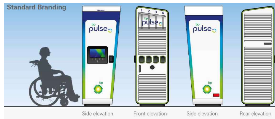
HYC400 Charger Standard Branding Elevations - Accessible NTS
