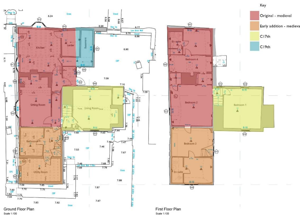
Fig 23: Existing Floor Plan showing Historic Development
