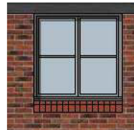
Canted Brick Cill
