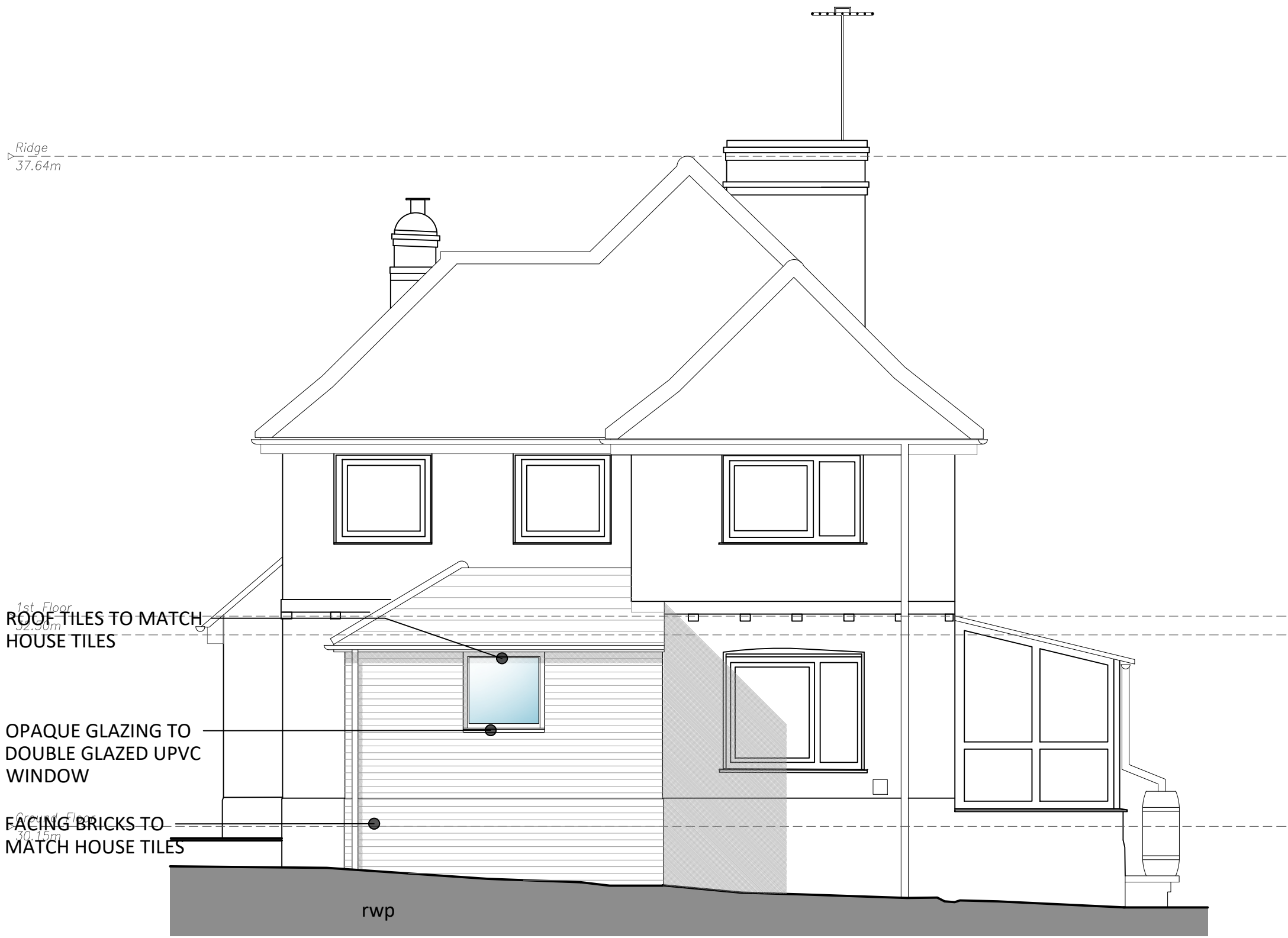
PROPOSED WEST ELEVATION
