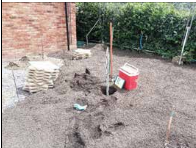
TS01 - Weald Clay Formation at Base of Excavation
