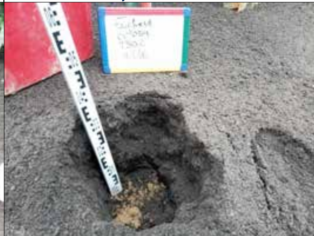
TS02 - Weald Clay Formation at Base of Excavation
