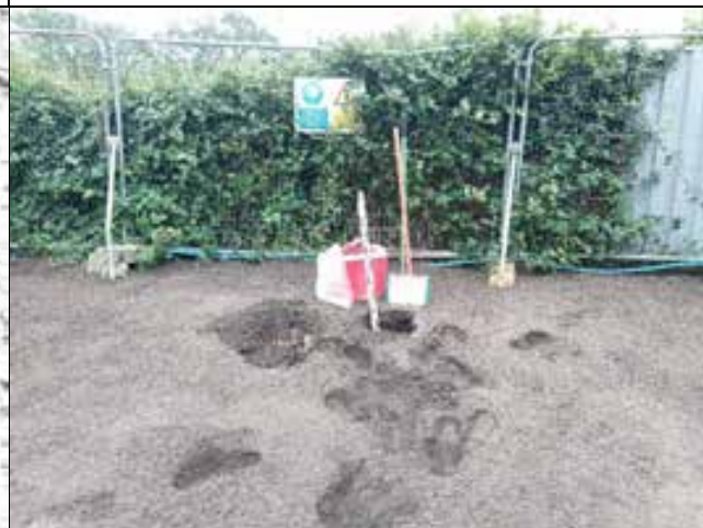
TS02 - Weald Clay Formation at Base of Excavation
