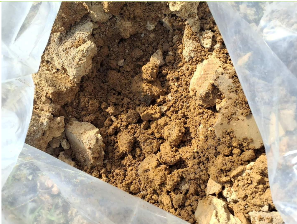
Plate 14 – Overview of slightly gravelly, silty sand of the weathered Hythe Formation from BH401.
