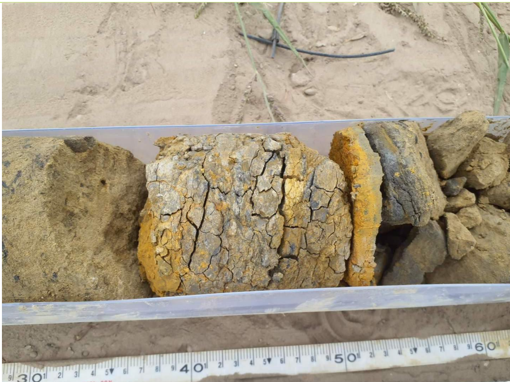
Plate 18 – Overview of horizon of dessicated clay within unweathered Hythe Formation in BH406
