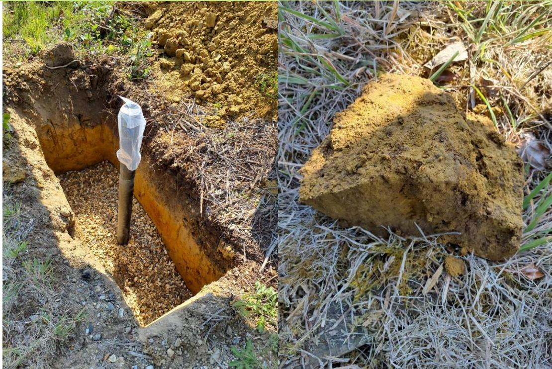
Plate 23 – Overview of SA401 installation (left) and sandy clay Head Deposit (right).
