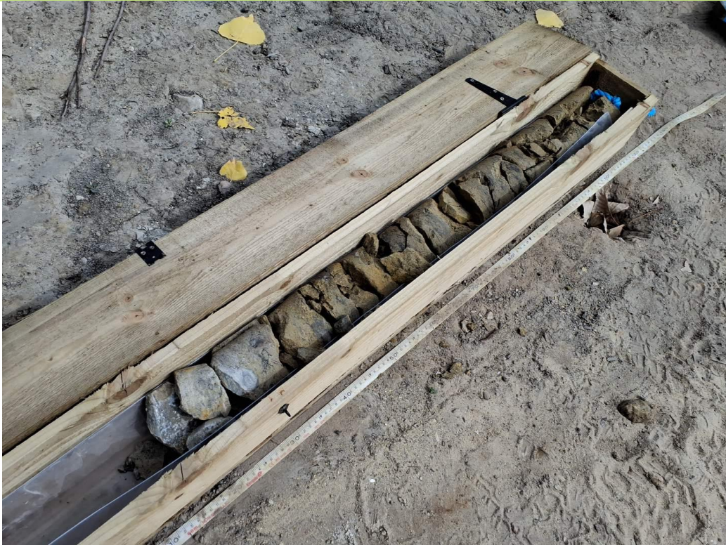
Plate 15 – Overview of interbedded limestone and sandstone in BH402
