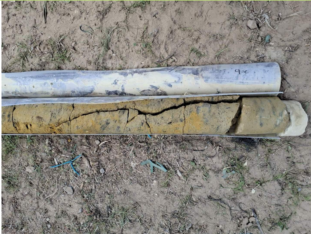
Plate 17 - Overview of sub-horizontal fracture in BH405
