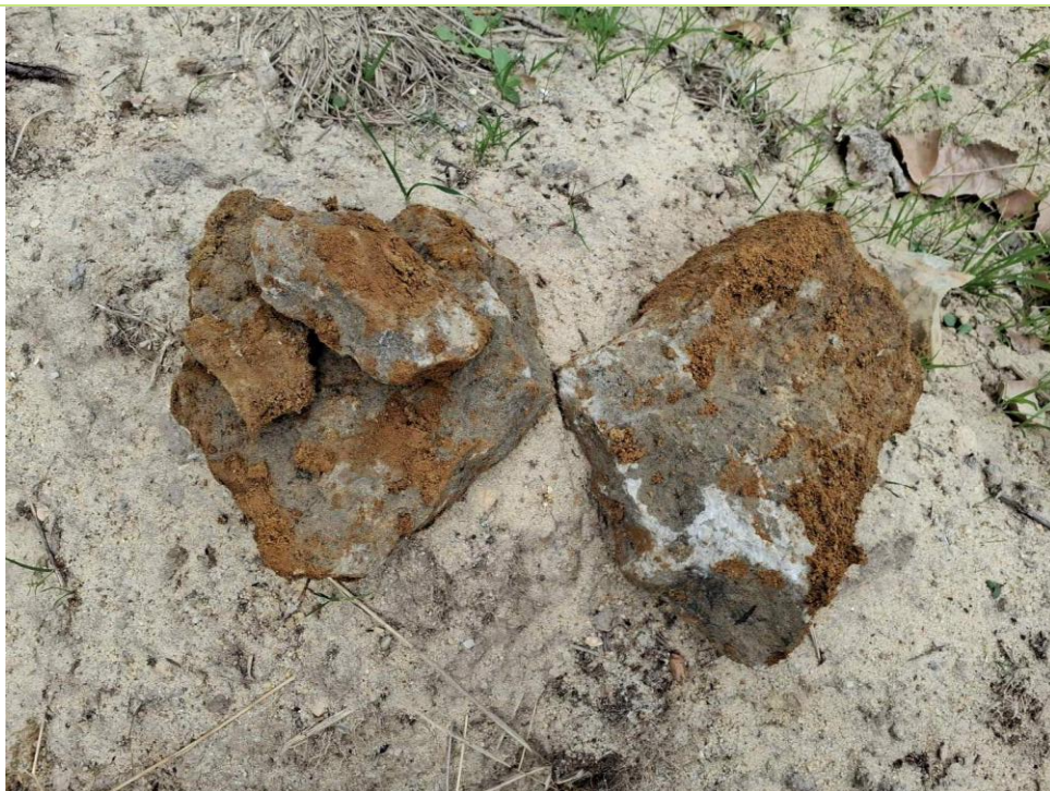
Plate 21 – Overview of topsoil and Hythe Formation from TP402
