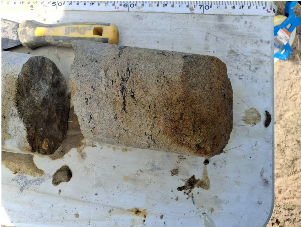
Plate 11 – Medium strong limestone from the Hythe Formation recovered from BH401.
