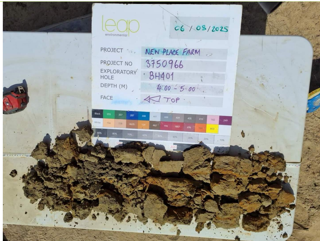
Plate 13 – Overview of weak sandstone from the Hythe Formation in BH401.
