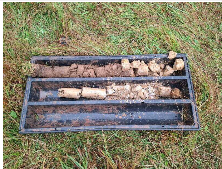
Photograph 6 – A view of an extracted window sample core (WS22)
