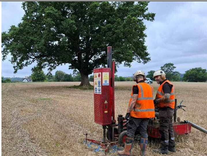
Photograph 1 – A view of a window sampling rig on position.
