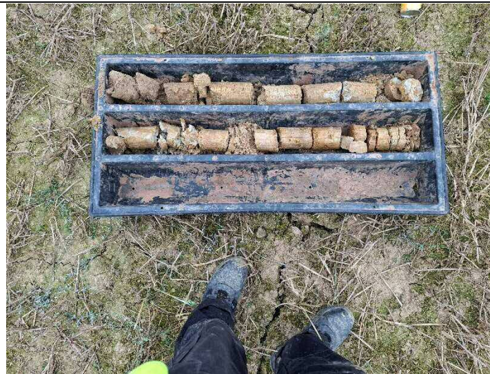
Photograph 2 – A view of an extracted window sample core (WS02).
