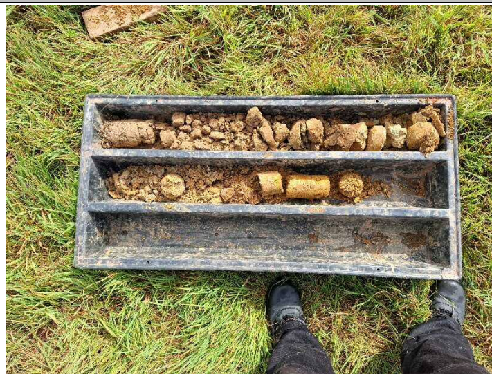
Photograph 4 – A view of an extracted window sample core (WS17).
