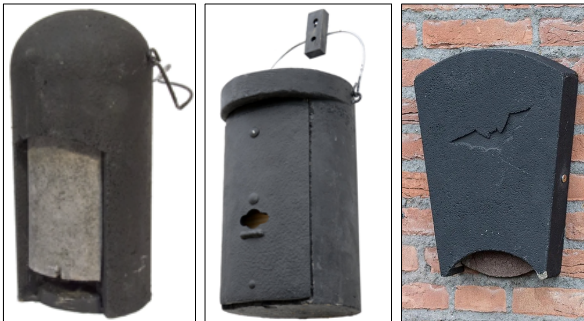
Figure 6. 2FN (left) and 1FS (right) bat boxes produced by Schwegler, and a Beaumaris Woodstone Bat Box (right). These and other brands are available at many online wildlife stores. These are constructed of a mixture of cement and woodchip and are designed to be durable and replicate the stable thermal properties of trees and buildings. They may be attached to trees or buildings.
