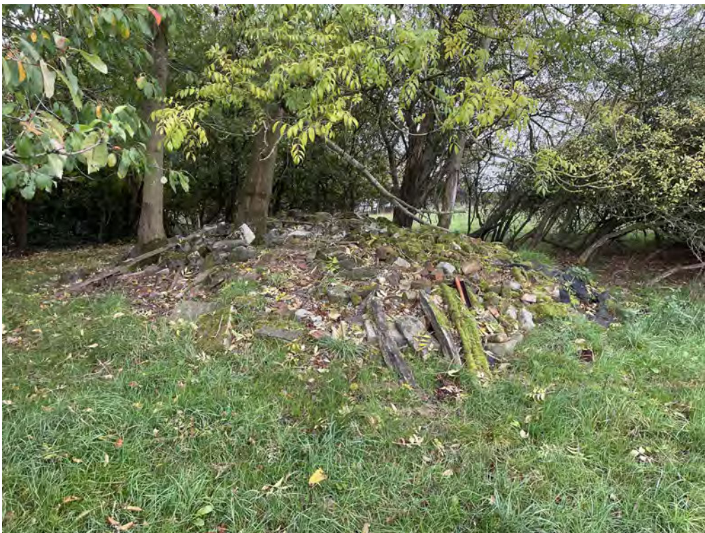
Photograph 2: View of stockpile 2, containing material of limestone brick, red brick, wood, asbestos sheeting, tile, ceramics, charcoal, asphalt, slate, glass, rubber, roofing, plastic piping, and concrete within the southwestern area of the site.
