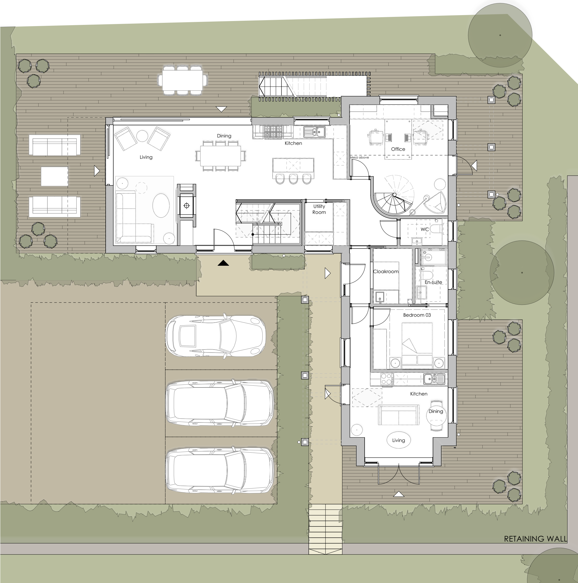
PROPOSED GROUND FLOOR PLAN 1:100@A1
