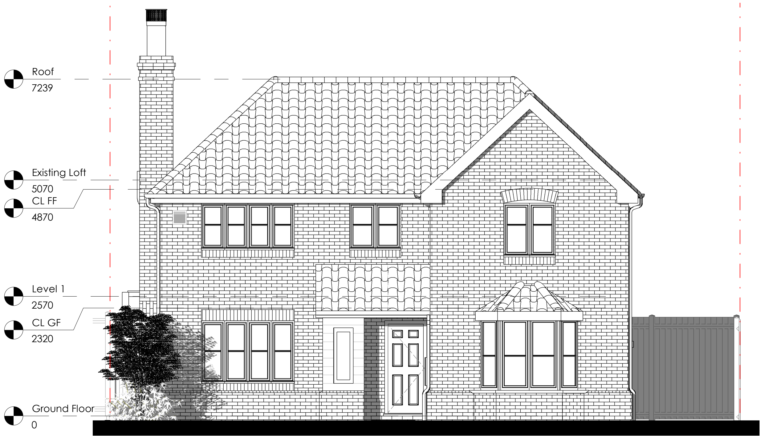
1 Existing Front Elevation 1 : 50
