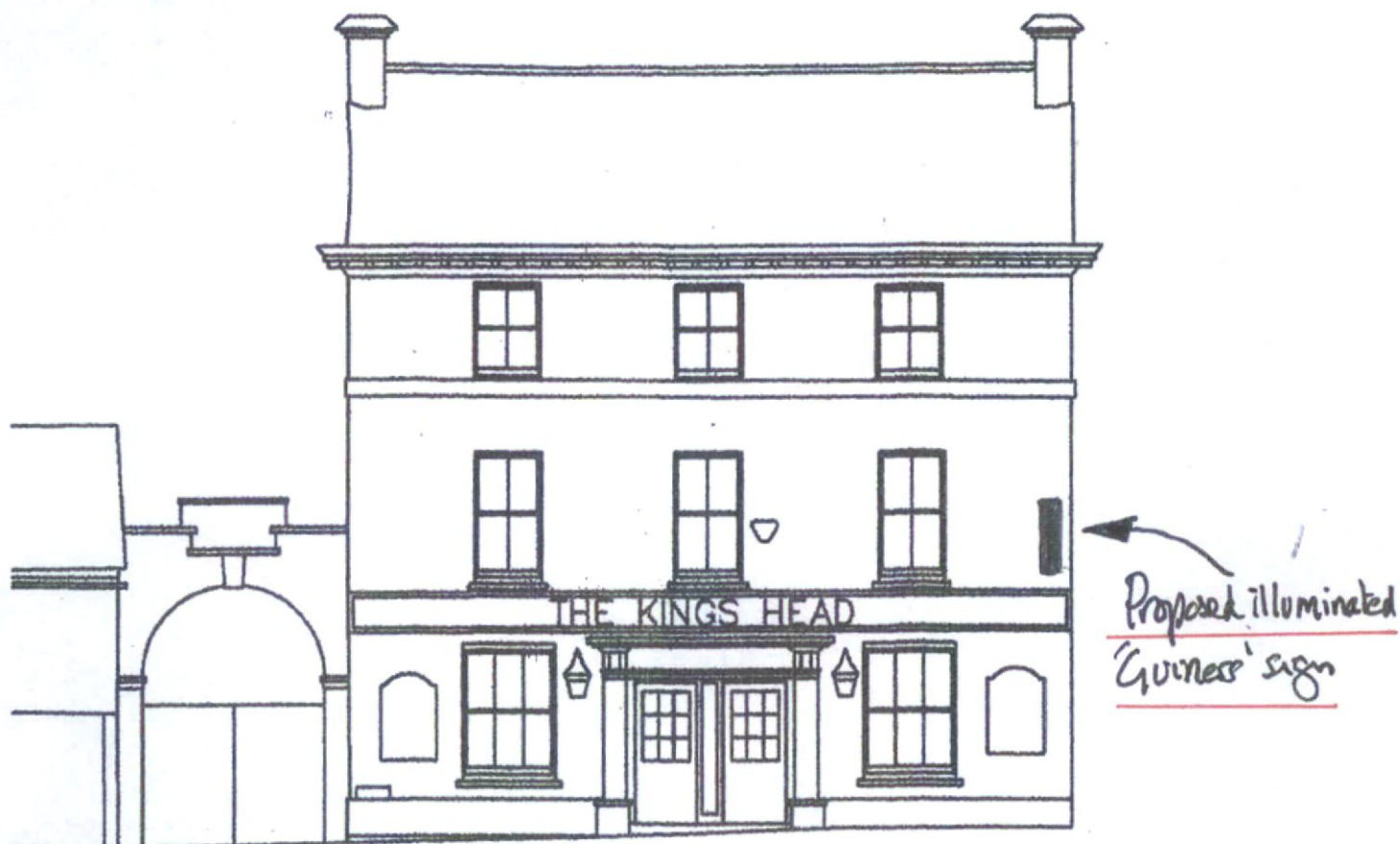
EXISTING EAST ELEVATION. [ FRONT ]
