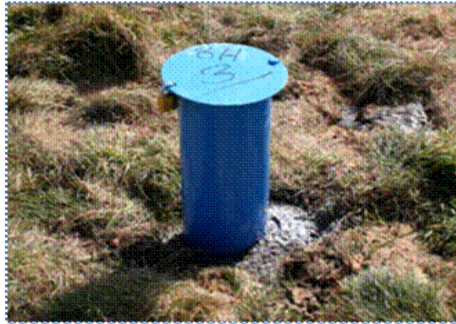
Figure 3 - Example Standpipe of GW survey borehole.
