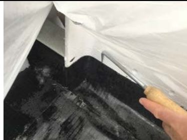
Probe testing the inner web of the steel stanchion detailing.
