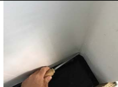
Probe testing the inner web of the steel stanchion.
