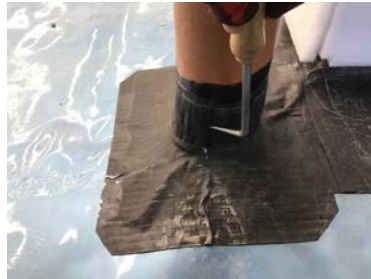
Probe testing a typical pipe penetration detail in unit 3.
