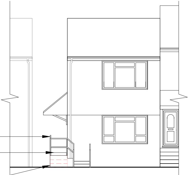
Existing front (north) elevation
