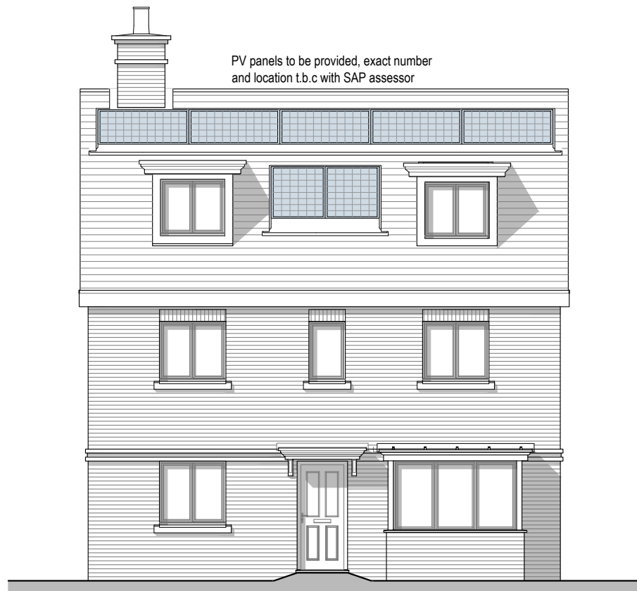
Front Elevation Chimney to plots 40, 152, 205 only
