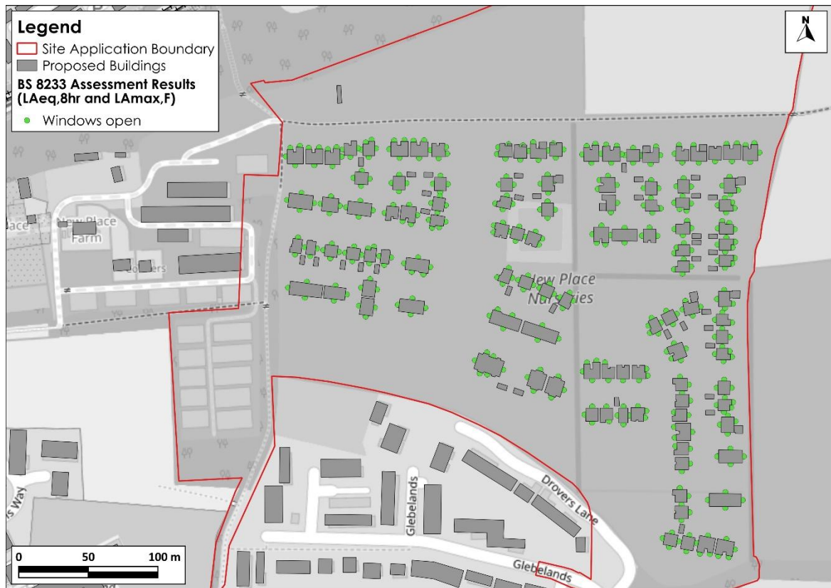
Figure 4-5: Night-time L_{Aeq,8hr} Internal Noise Level Assessment
