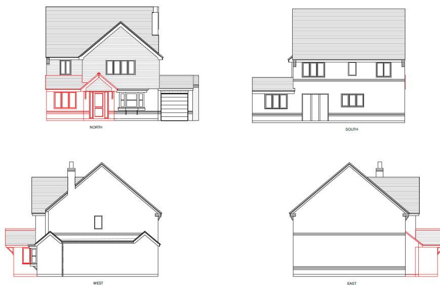
Figure 4 Proposed Elevations new works lined in red
