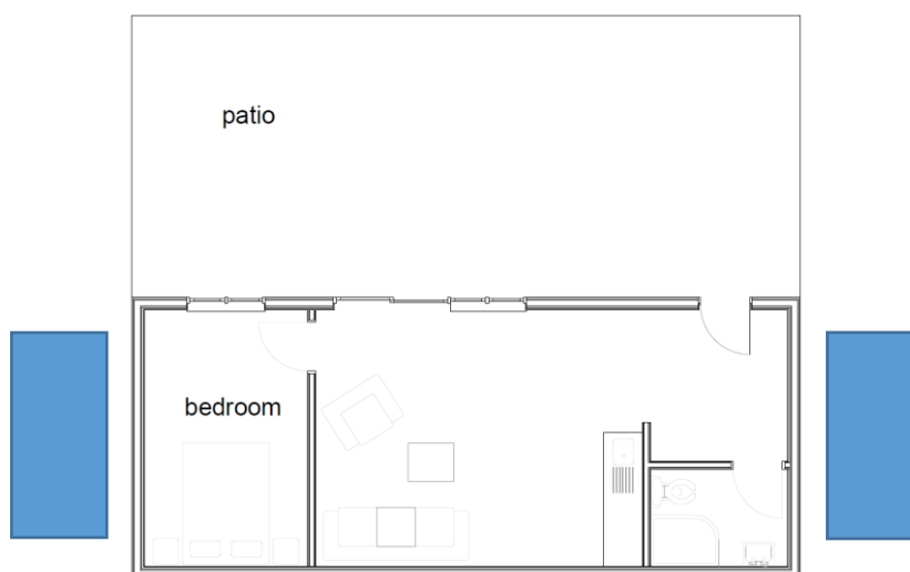
Fig. 4 Potential Rainwater Harvesting tank locations
