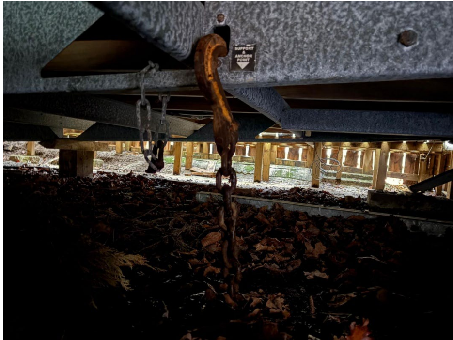
Figure 3.3 – Photo Showing Caravan Attached to Ground
