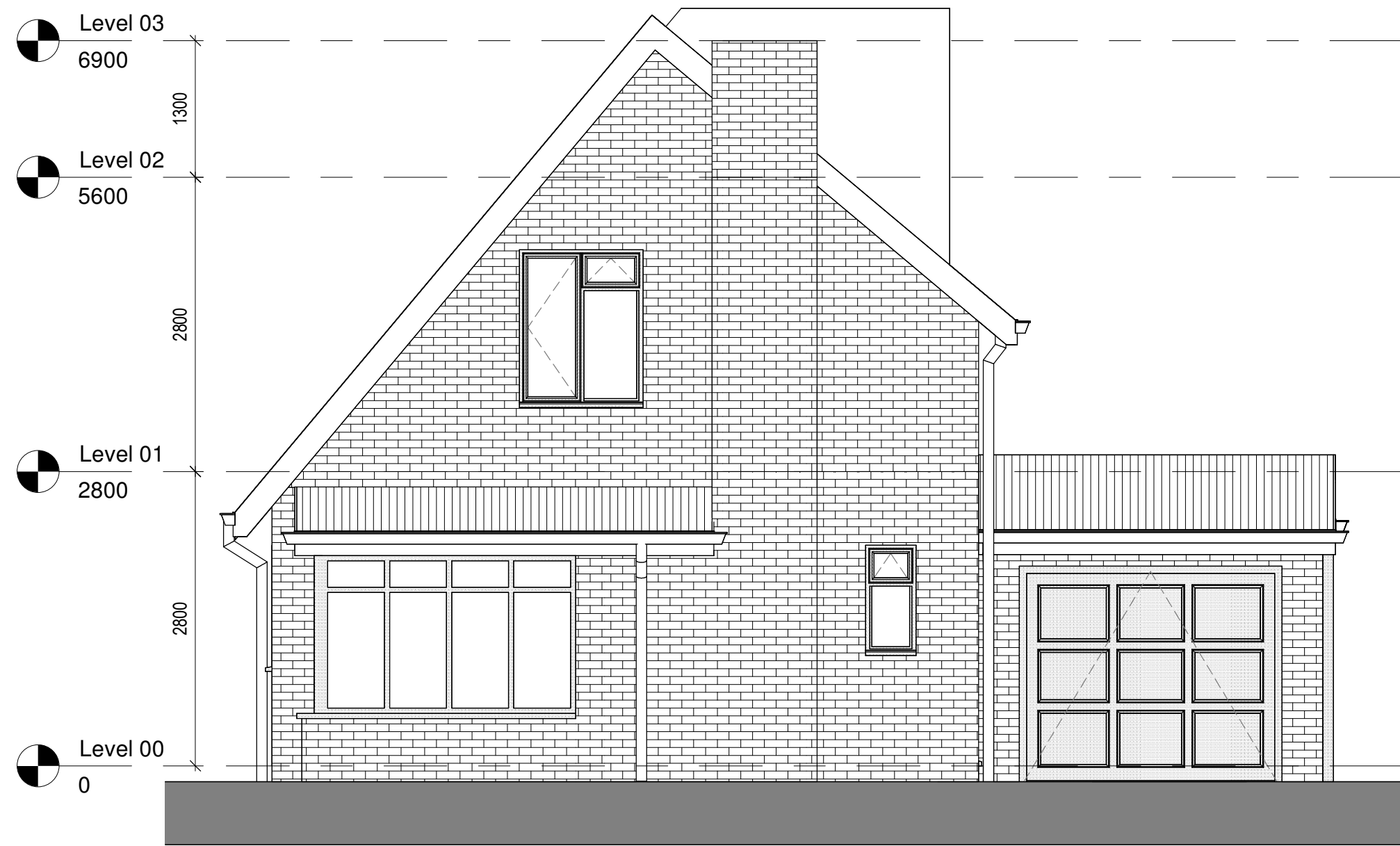
1 Front Elevation - Existing 1 : 50
