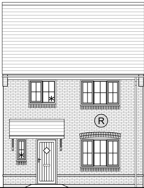
FRONT ELEVATION AS: 54, 59, 73, OPP: 58, 72, 82 * Obscure glazing
