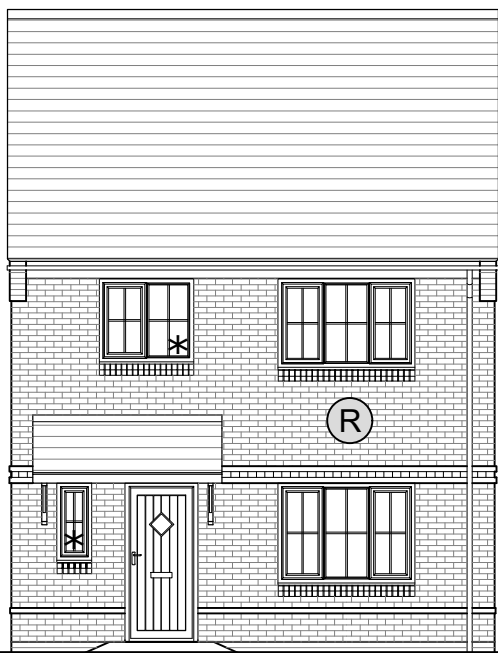
FRONT ELEVATION AS: 52, 78 OPP: 23, 51 * Obscure glazing
