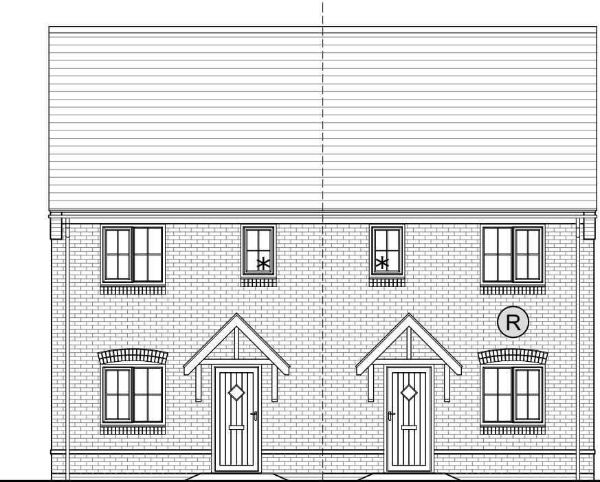
FRONT ELEVATION As: 48-49, 55-56 * Obscure glazing
