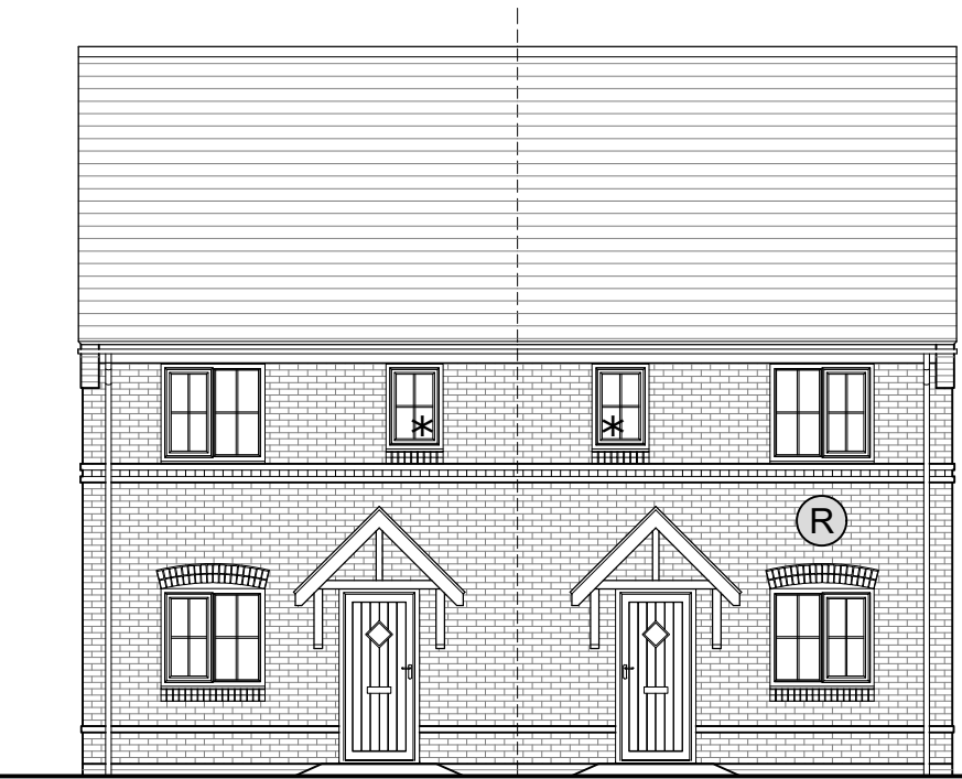
FRONT ELEVATION As: 44-45, 79-80 * Obscure glazing
