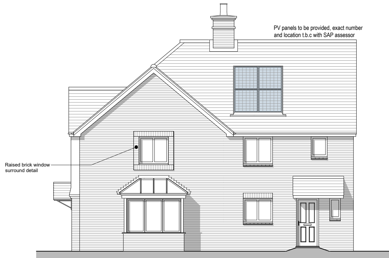
Front Elevation No chimney to Plots 202-203
