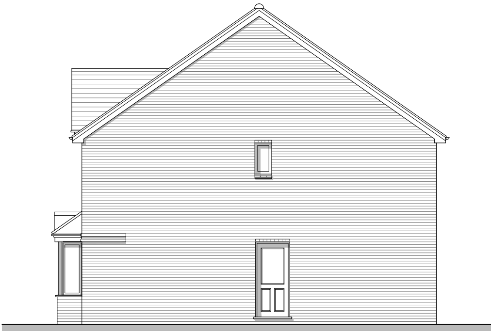
Side Elevation Chimney (shown dotted) to Plot 95 only
