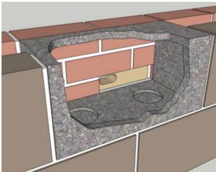
Figure 30. A schematic of how the Cambridge full face Swift brick leads into a cavity created by the prior installation of the Swift maxi nesting box.
