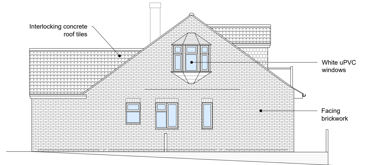
EXISTING SIDE ELEVATION
