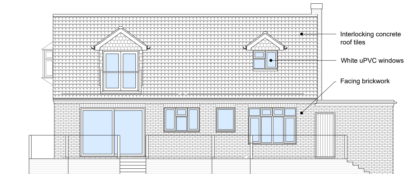
EXISTING REAR ELEVATION
