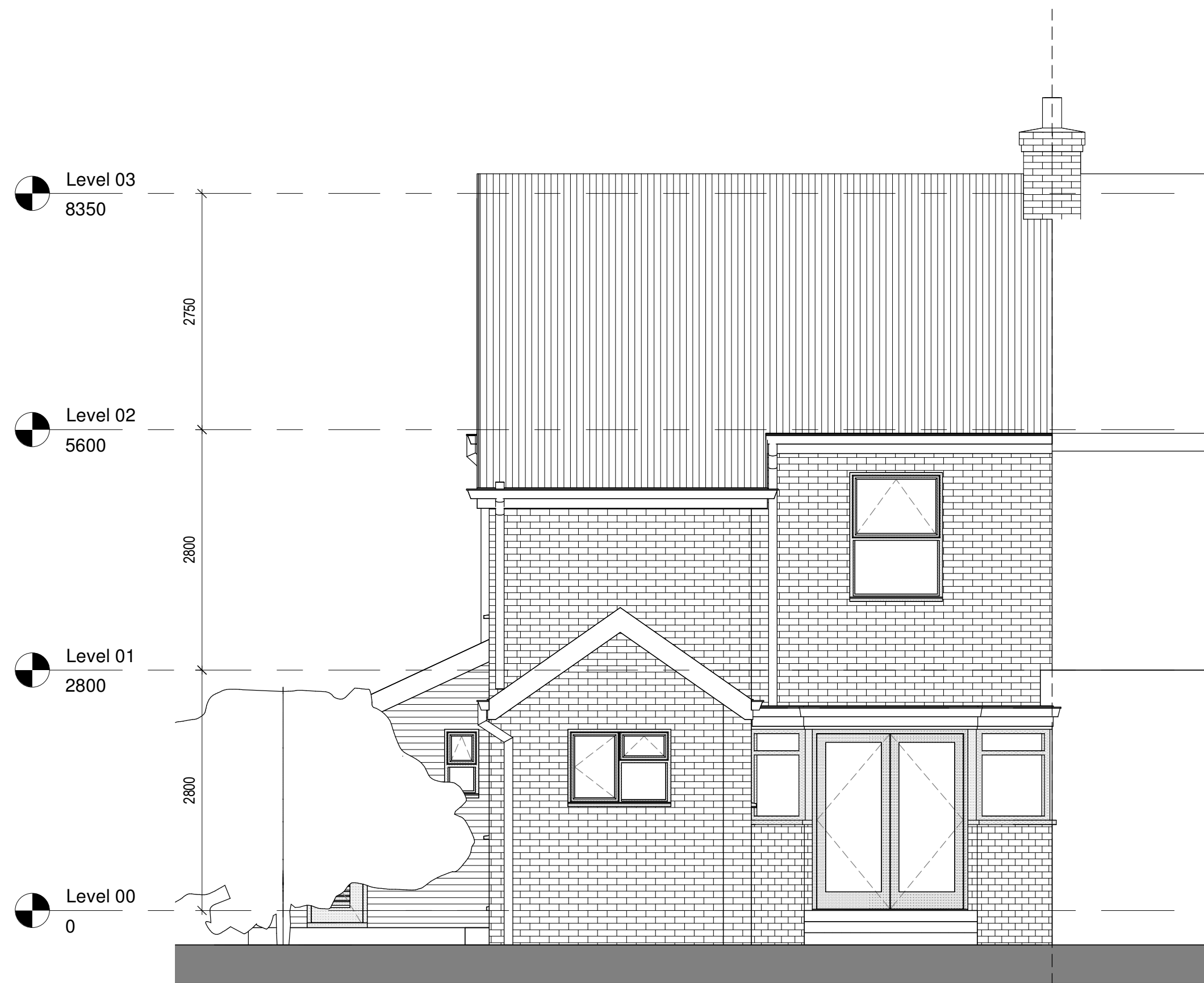
3 Rear Elevation - Existing 1 : 50
