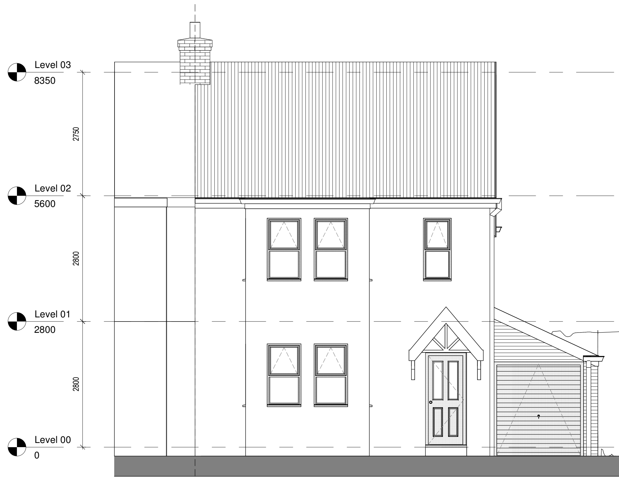
1 Front Elevation - Existing 1 : 50
