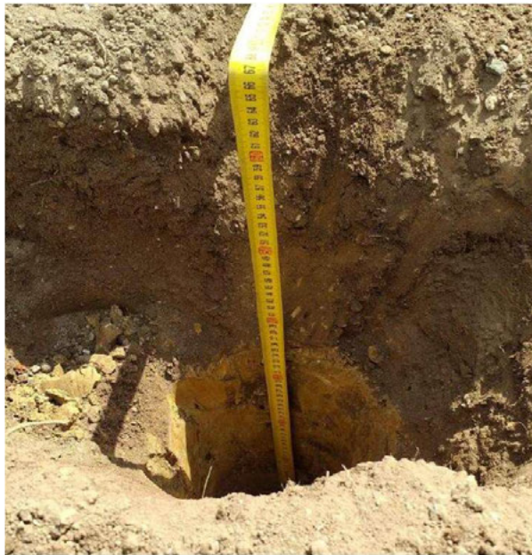
Inspection Pit in Plot 4 showing 400mm of Topsoil and Formation Soils Beneath
