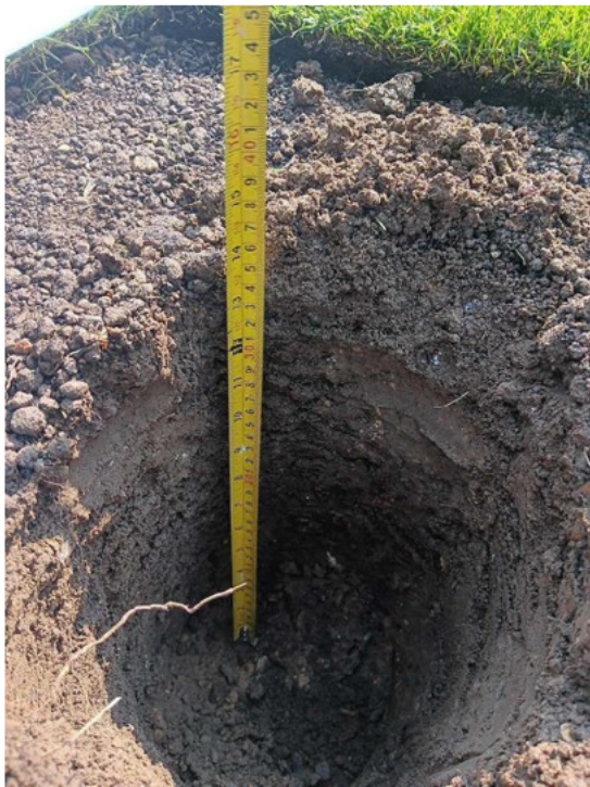
Clean cover in Plot 7 showing ~350mm of topsoil
