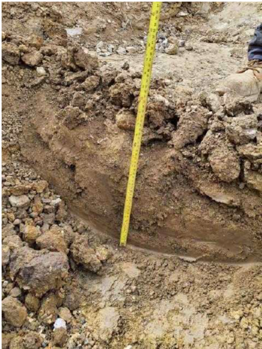
Pit excavated into formation level of Plot 7
