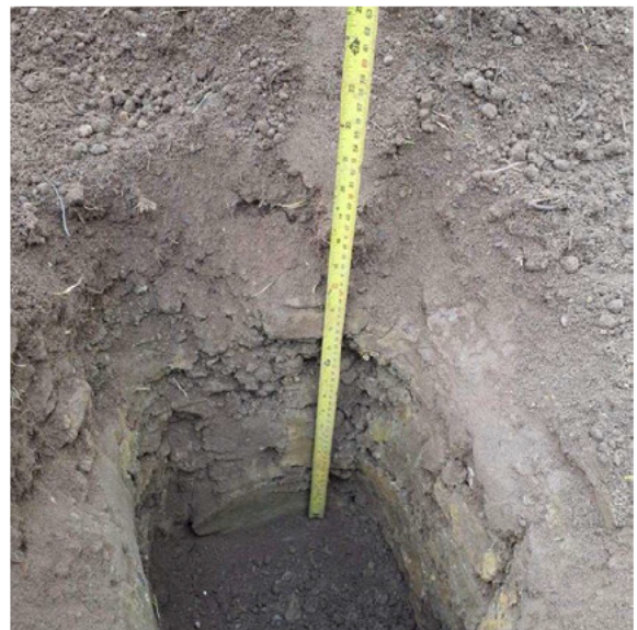
Inspection Pit in Plot 2 showing thickness of clean cover
