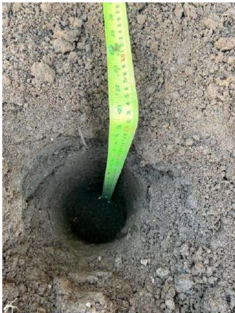
Inspection pit (Apart-2) in Apartment block area on 28 th October 2025 showing 450mm of Topsoil
