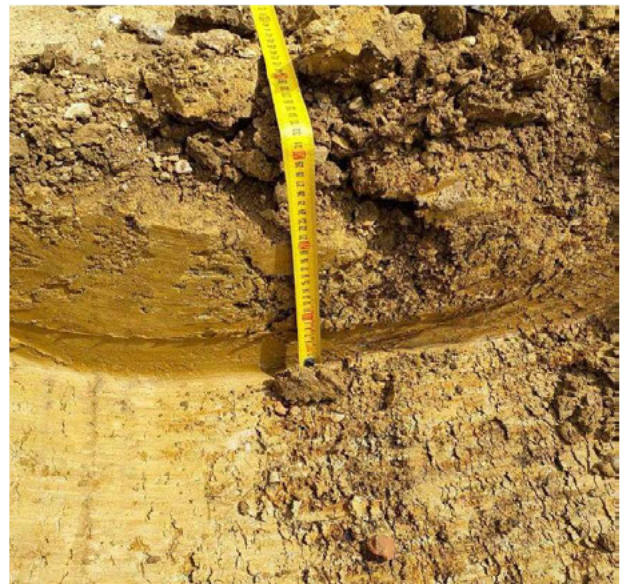
Inspection pit excavated 300mm below formation level to evidence natural clay in Plot 4
