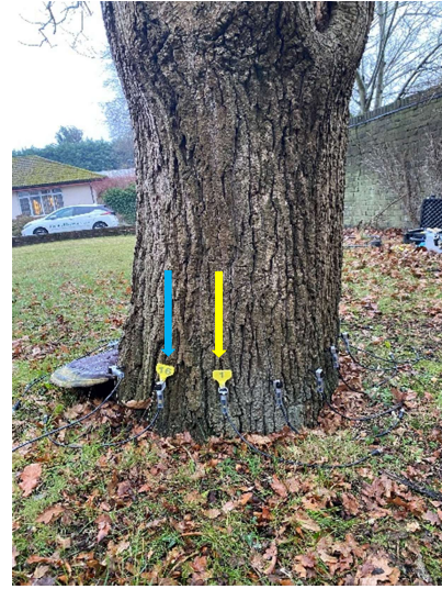
Photo 2. SOT sensor positions looking South Yellow arrow = sensor 1 at North Blue arrow = sensor 16
