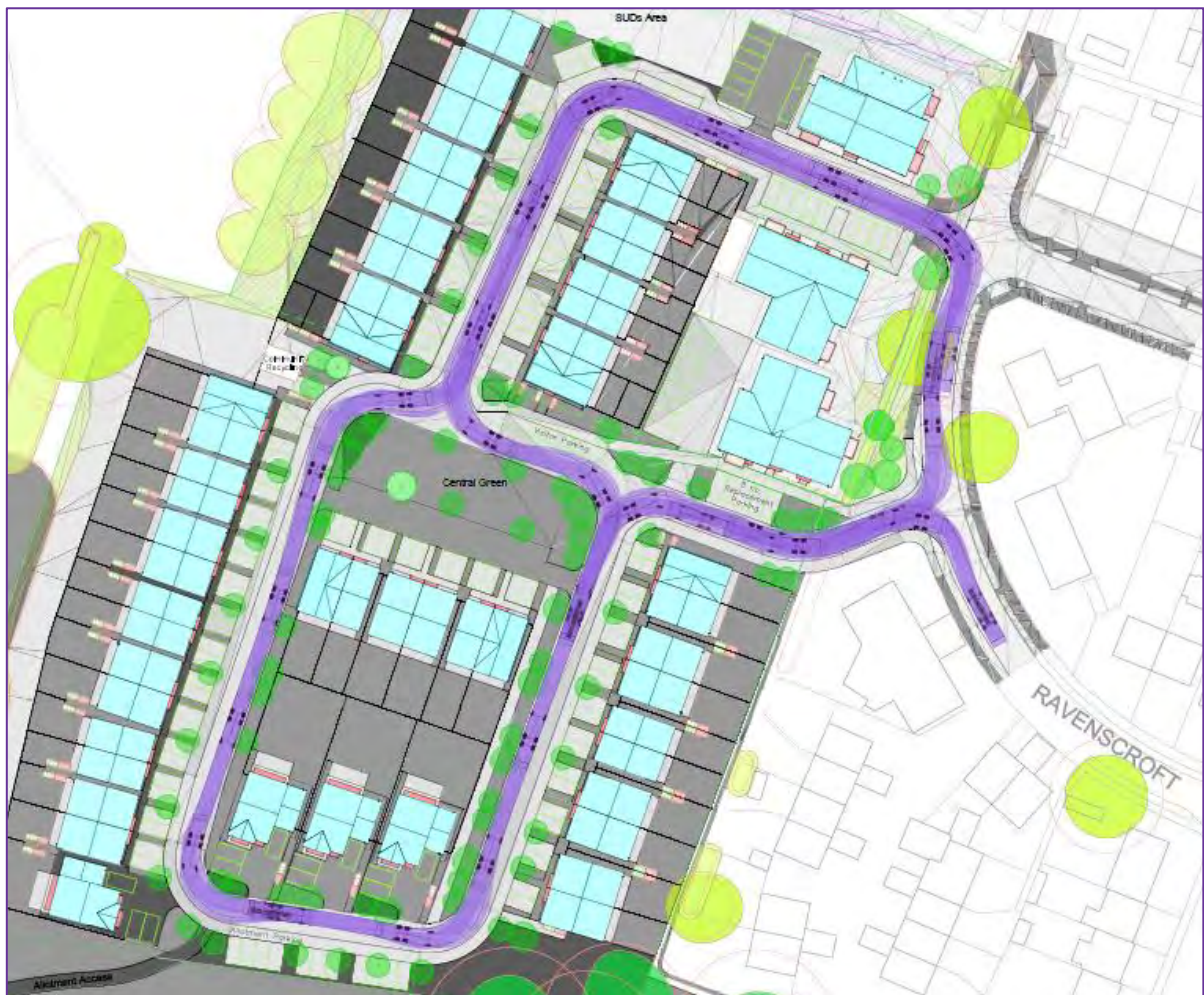
Image 3.2: Swept Path Analysis: Refuse Vehicle
