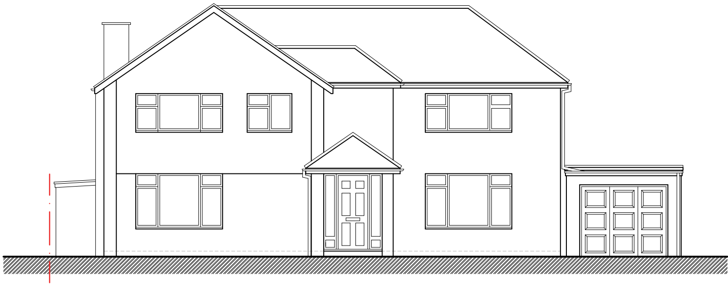
FRONT ELEVATION EXISTING ELEVATIONS SCALE 1:100
