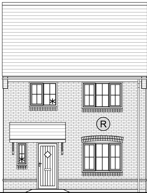
FRONT ELEVATION AS: 54, 59, 73, OPP: 58, 72, 82 * Obscure glazing
