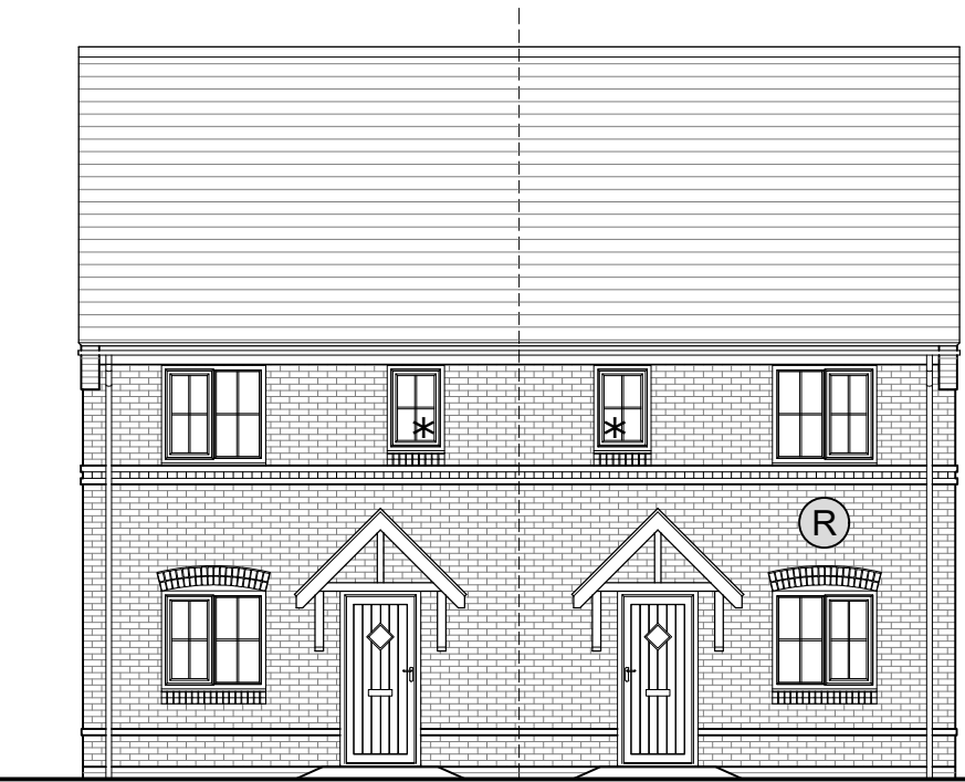
FRONT ELEVATION As: 44-45, 79-80 * Obscure glazing
