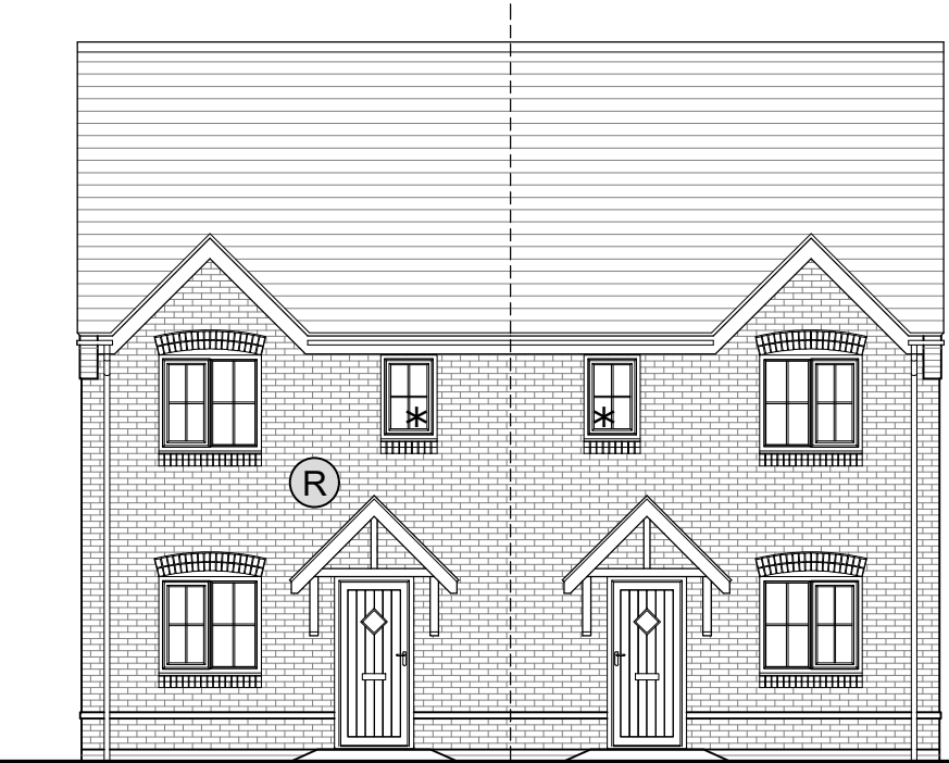
FRONT ELEVATION As: 48-49, 55-56 * Obscure glazing
