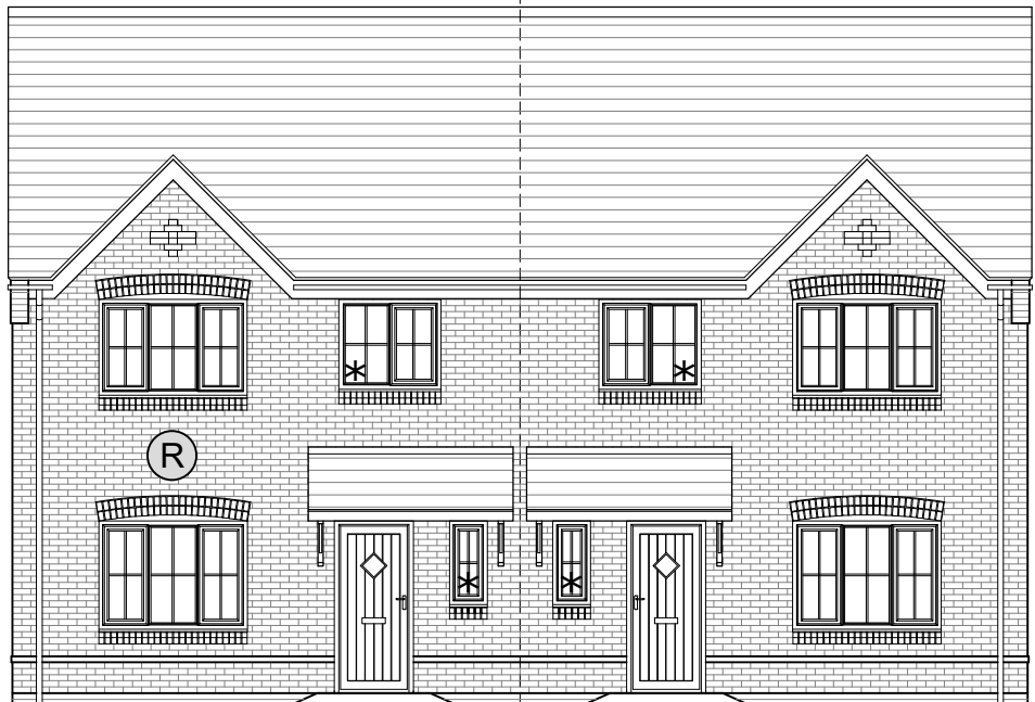
FRONT ELEVATION As: 27-28 Handed: 25-26 *Obscure glazing
