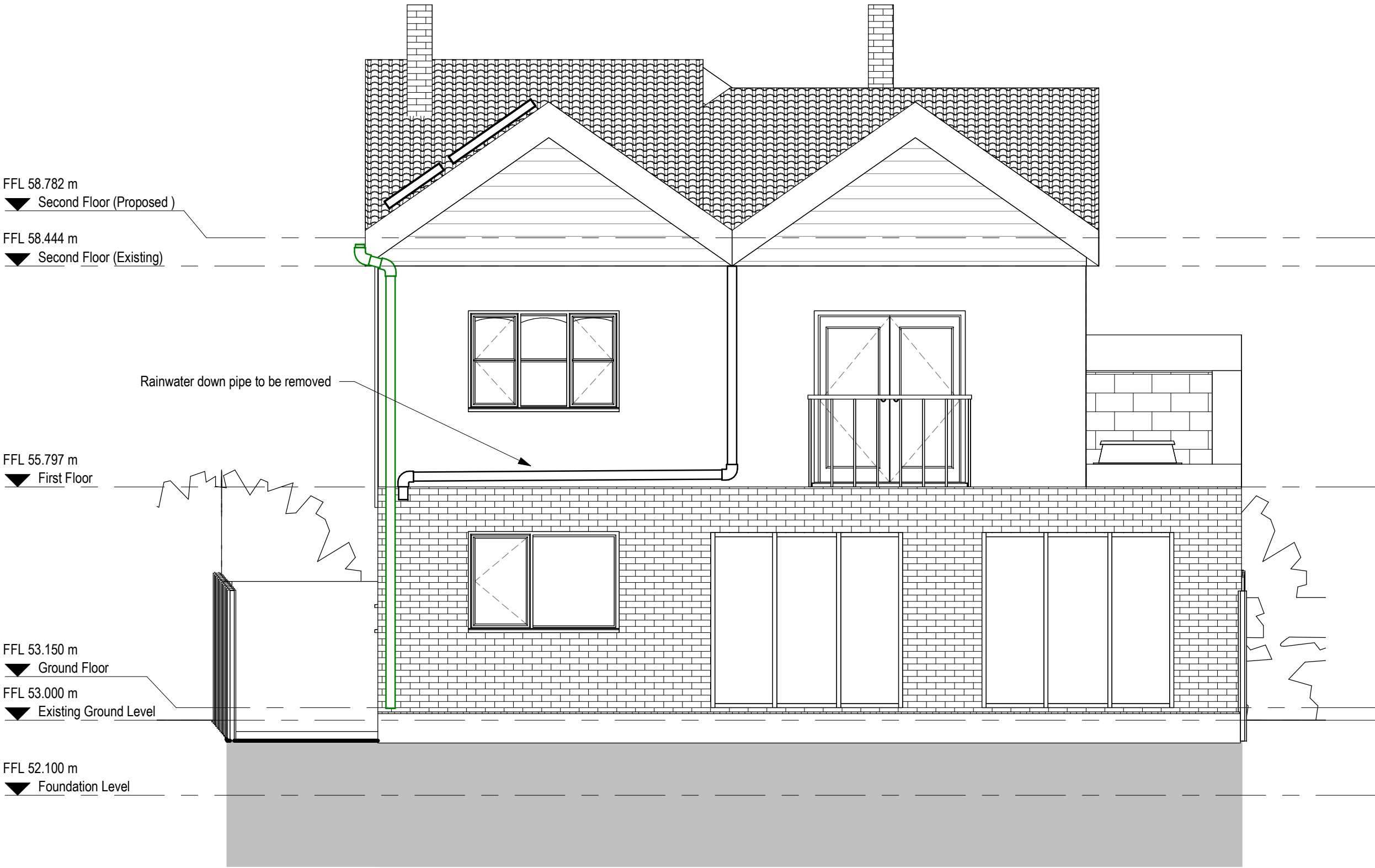
1 East Elevation (Existing) 1 : 50
