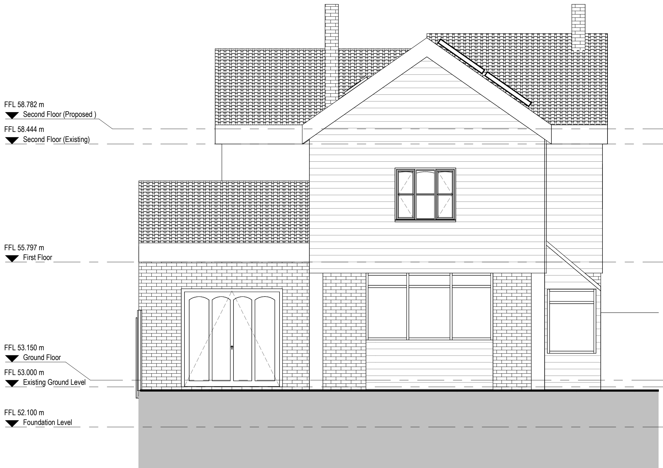
4 West Elevation (Existing) 1 : 50
