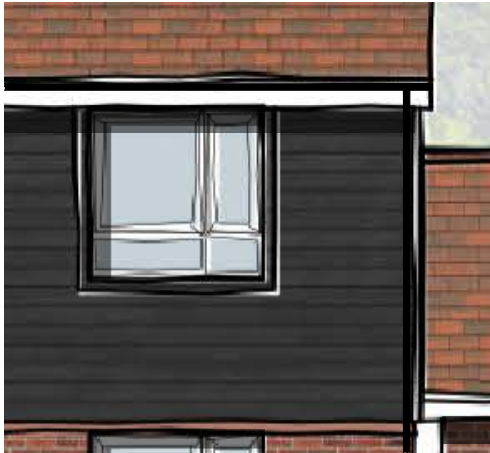
Black Weatherboarding and Metal Frame
